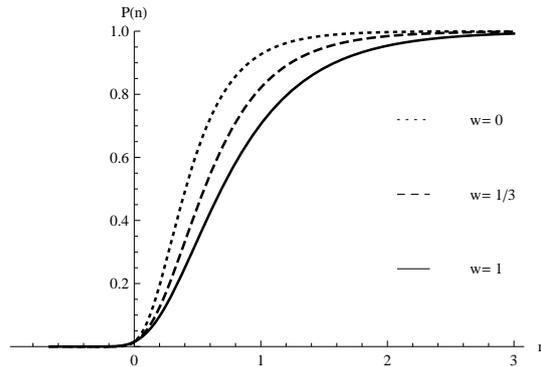
Figure 4: Tunneling probability (40) for the model with varying  $c$  ( $k = +1$ ,  $q = 0$ ,  $\Lambda = 5$ ,  $\hbar = G_0 = c_0 = 1$ ) for three different cases: the universe filled with dust ( $w = 0$ ), radiation ( $w = 1/3$ ) and stiff fluid ( $w = 1$ ). In the scenario with diminishing  $c$  ( $n < 0$ ) the tunneling probability is much lower than the tunneling probability in the scenario with  $c$  growing ( $n > 0$ ).
